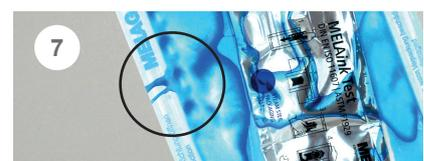
The ink test has been failed - the ink has revealed a channel in the seal seam.
